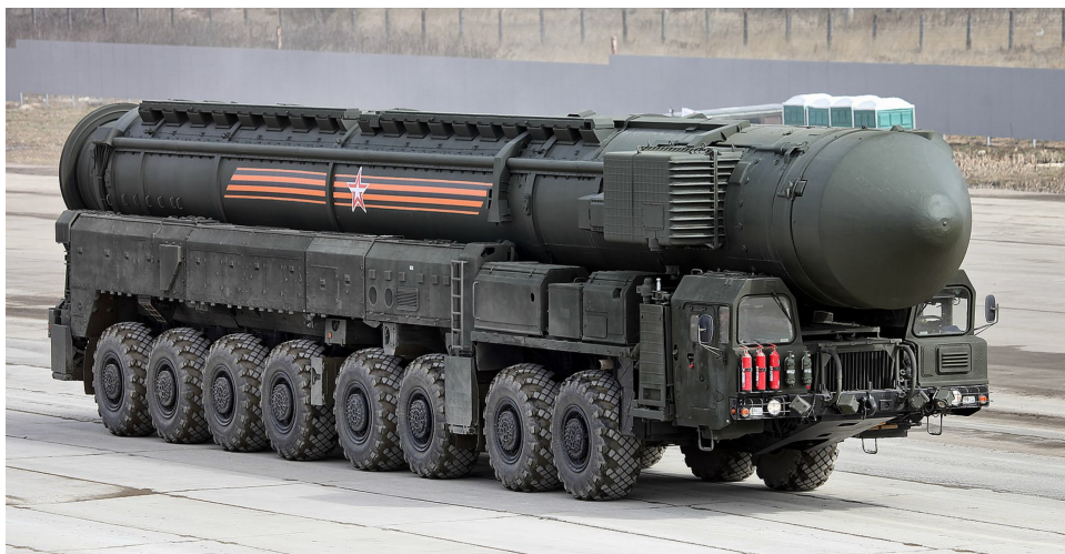
A Russian RS-24 Yars, a vehicle for deploying a nuclear ICBM (intercontinental ballistic missile).
